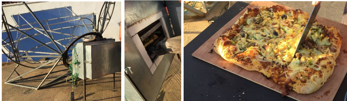
Figure 2. Solar concentrating system in Tamera community: a) view of overall system, b) chamber with sensible storage medium and c) pizza.
