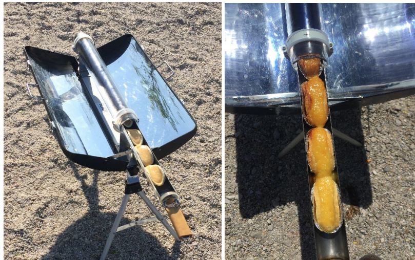
Figure 2. Evacuated tube solar cooker baking Portuguese custard tarts (pastéis de nata): a) starting and b) final baking result.
