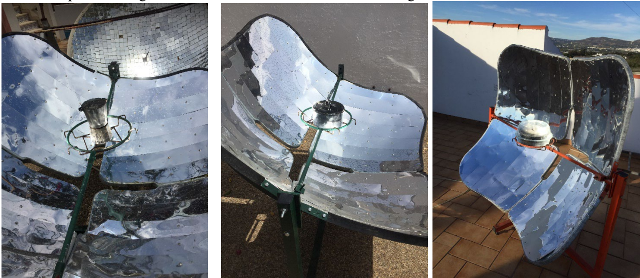
Figure 1. Parabolic solar cooker PRINCE15 with different cooking vessel: a) Italian coffee maker, b) black pot and c) set of glass enclosure and black pot.
